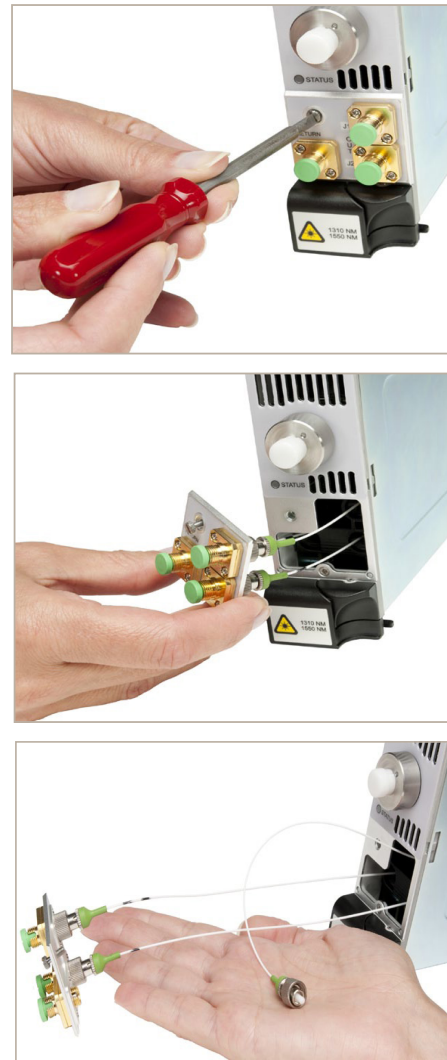
Step-by-step example of opening the front panel door to maintain the launch connectors
